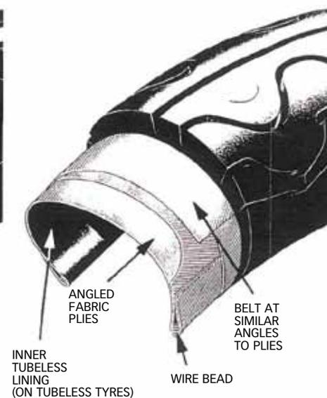
Depending on the wheel type, these may be tubeless (no tube required); or tube type (requiring an inner tube).
