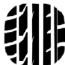
CONTACT WITH ROAD EVEN ACROSS TREAD WIDTH
