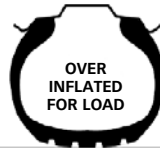
CONTACT WITH ROAD IN CENTRE OF TREAD
