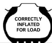
CONTACT WITH ROAD EVEN ACROSS TREAD WIDTH
