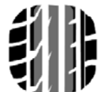
CONTACT WITH ROAD CONCENTRATED ON TREAD EDGES
