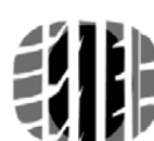
CONTACT WITH ROAD IN CENTRE OF TREAD
